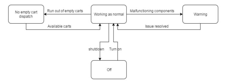
The control system features three working states and one off state. The control system is typically in the "working as normal" state for most of the time. "Warning" and "no empty cart dispatch" are states of concern indicating a deficiency in the running system, these issues should be promptly resolved to avoid further inefficiencies or damages. The system will attempt to continue to work during states of distress.
