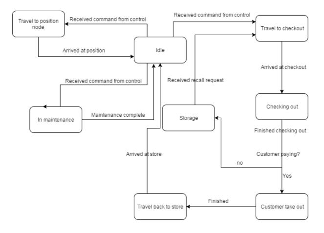
The cart can be in a number of different states. The states are changed in response to commands received and context such as current state. Idle is the state the cart is most often in. Idle state allows for actionable responses to commands received from the control center. A cart will experience all the states multiple times during its typical lifecycle.
