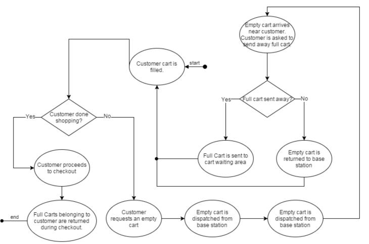
The activity diagram above shows the expected flow that customers will take during their interaction with the system. Because it is expected that all users will enter and exit the store at some point, there are entry and exit points marked "start" and "end" that designate when the user enters or exits the store. In addition, the pictorial representation of the expected flow for the customer does not take into account potential errors that the system occurs, and assumes the "happy path".
