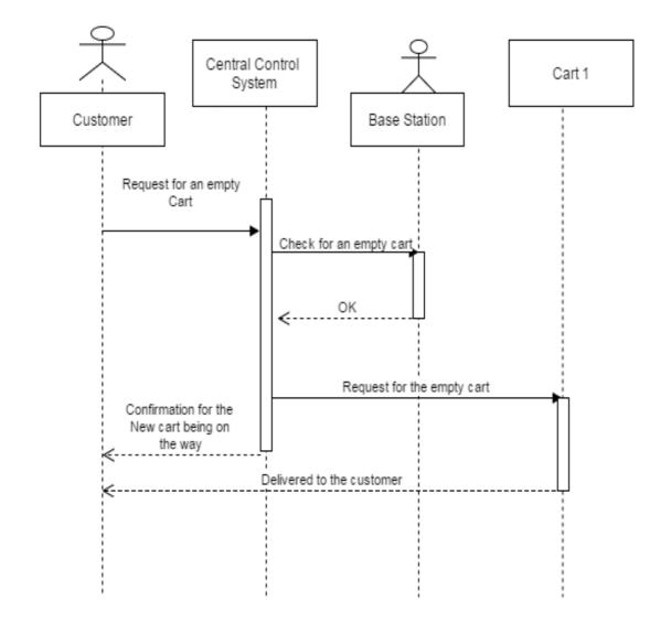
The customer requests for an empty cart from a particular location. The Central Control System gets the requests and checks if there are any empty cart in the base station. The base station returns an OK signal. The Central Control System requests an empty cart, and confirms the customer about the empty cart being on the way. In the meantime, the requested empty cart goes to the customer's location. Sequence diagram for switching carts
